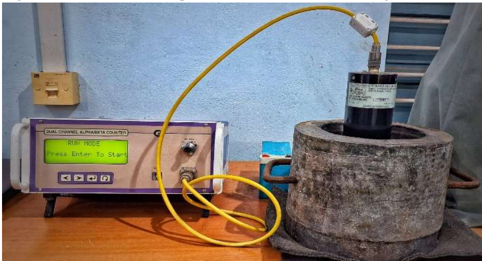
Figure.2. The dual channel alpha, beta counter used for counting
